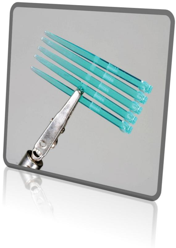
With a gate diameter of 0.8 mm all articles filled completely right after re-starting the mold with the first shot again. There was no evidence of stringing or drool of the plastic.
