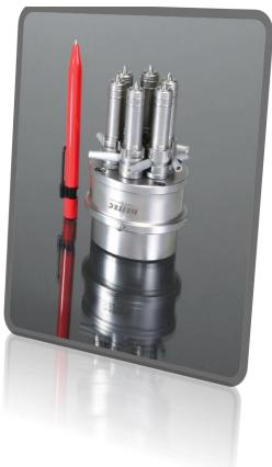
Thanks to the highly precise, thermal profile of the nozzle, it was possible to obtain a very small injection point diameter of 0.32 mm. The injection point received a very high rating and the outlines were optimal. As manifold of the 4-fold application, the distributor nozzle also known as a rotary distributor, was
